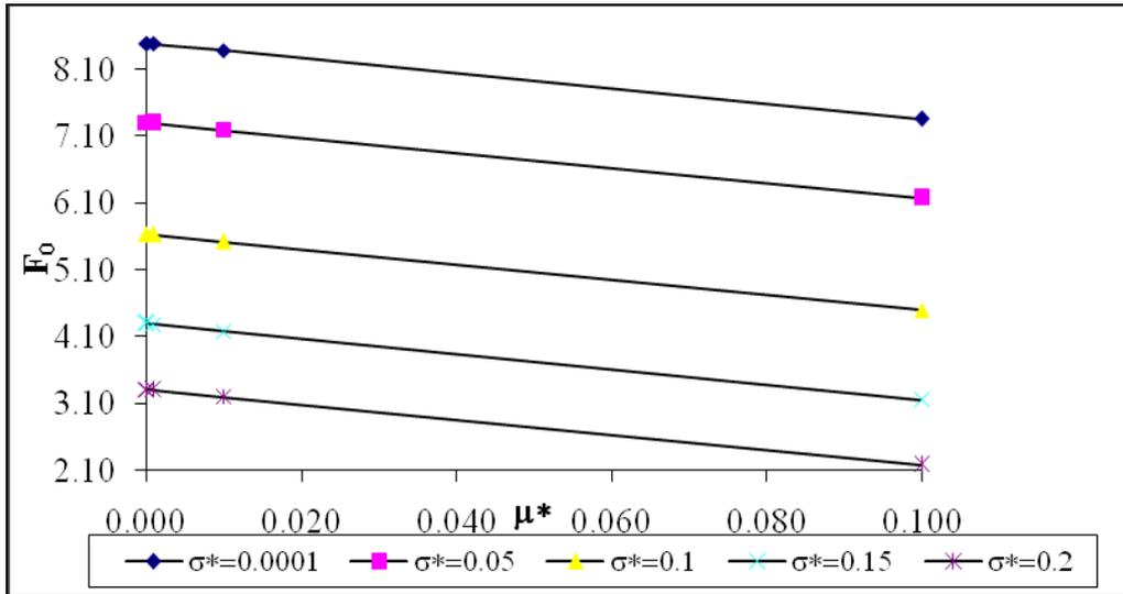
Fig. 7 Variation of frictional force at moving plate with respect to  $\mu^*$  and  $\sigma^*$ .
