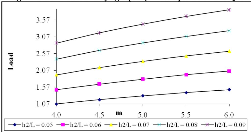
Fig. 6 Variation of load carrying capacity with respect to  $m$  and  $h_2/L$ .
