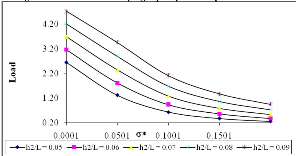
Fig. 5 Variation of load carrying capacity with respect to  $\sigma^*$  and  $h_2/L$ .
