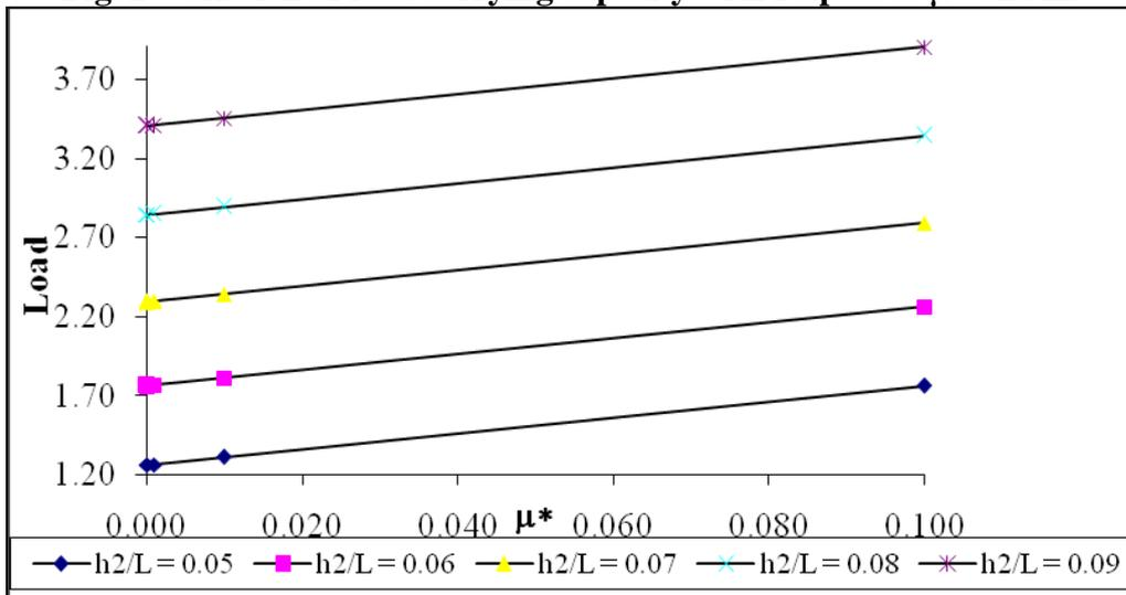
**Fig. 3** Variation of load carrying capacity with respect to  $\mu^*$  and  $h_2/L$ .
