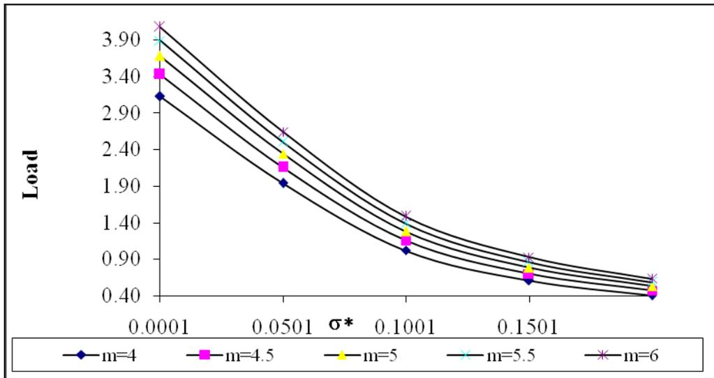
Fig. 4 Variation of load carrying capacity with respect to  $\sigma^*$  and  $m$ .
