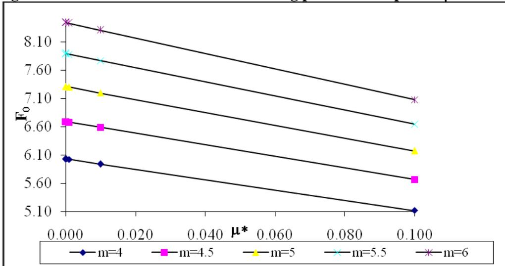
Fig. 8 Variation of frictional force at moving plate with respect to  $\mu^*$  and  $m$ .
