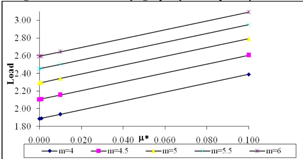
**Fig. 2** Variation of load carrying capacity with respect to  $\mu^*$  and  $m$ .
