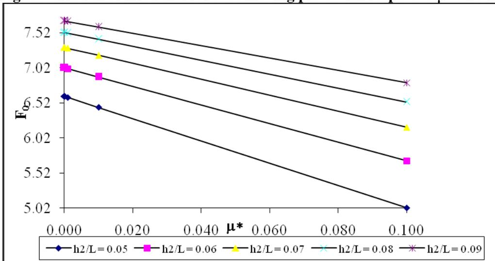
Fig. 9 Variation of frictional force at moving plate with respect to  $\mu^*$  and  $h_2/L$ .
