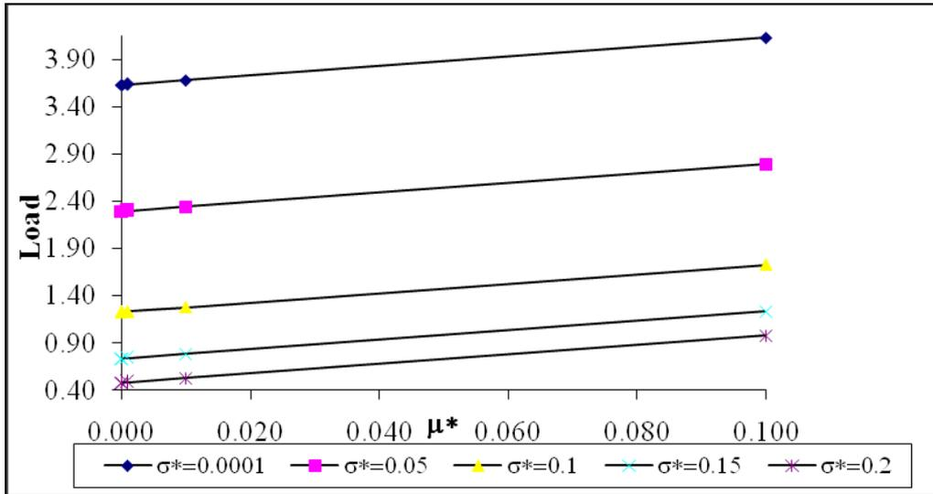
**Fig. 1** Variation of load carrying capacity with respect to  $\mu^*$  and  $\sigma^*$ .
