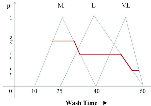
Since output Wash Time should be a crisp value, defuzzification procedure is required.
