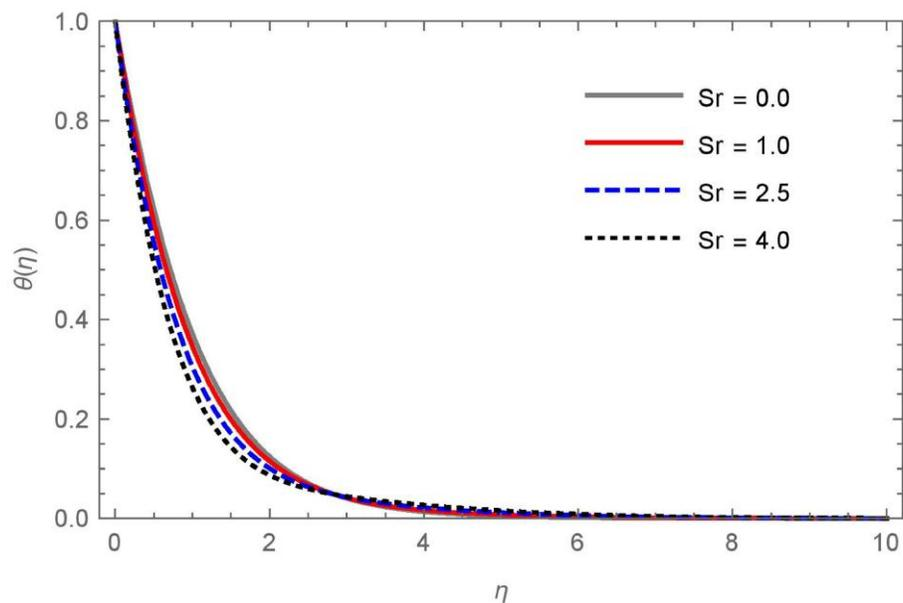
**Figure 8: Temperature Profile for Different value of  $Sr$**
