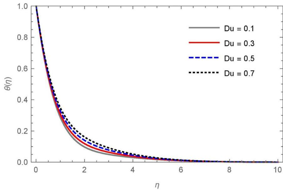
**Figure 6: Temperature Profile for Different value of  $Du$**
